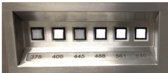
Figure 4-2 Laser power panel
