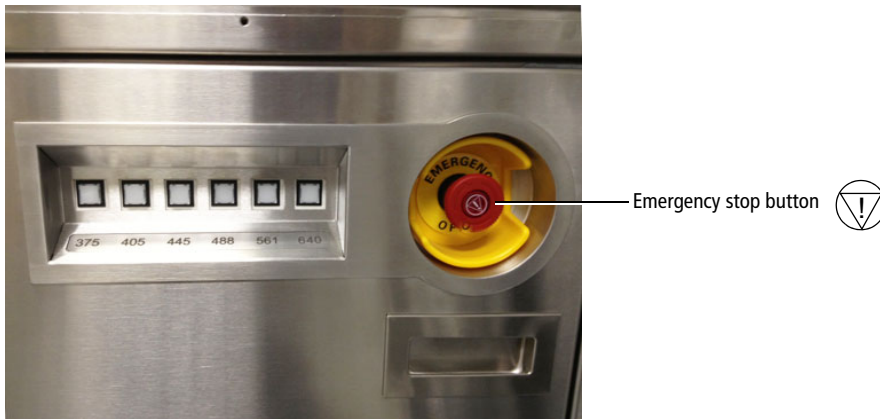
Figure 1-25 Emergency stop button
