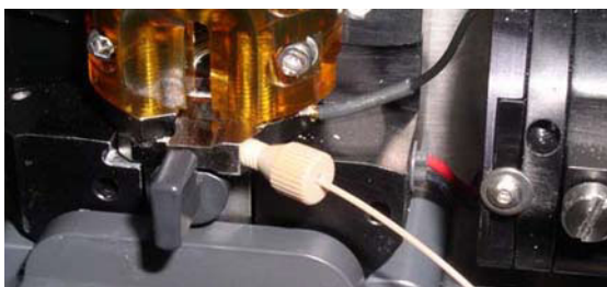
Figure 6-1 Closed-loop nozzle installed in flow cell
