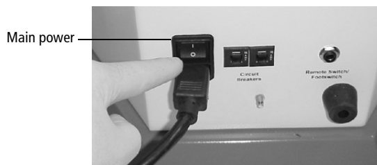
Figure 10-4 Turning on main power
