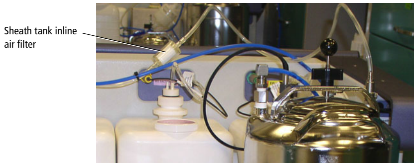
Figure 6-15 Inline air filter for sheath tank
