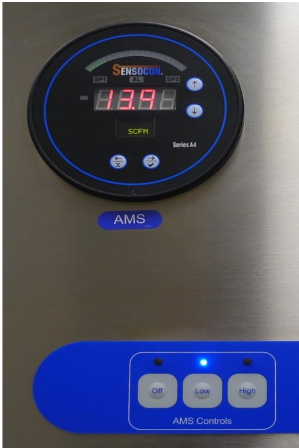
Fig. 9 Aerosol Management System Control Panel
