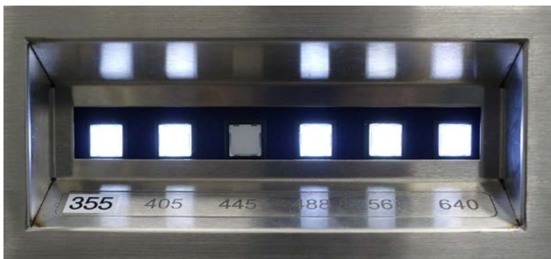
Fig. 3 Laser Power Panel
